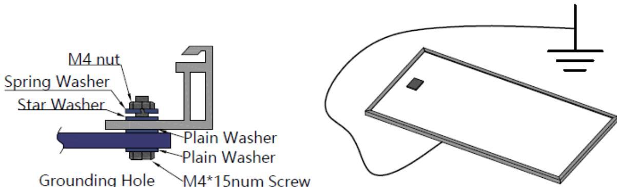
Figure 10.2: Ground installation of PV modules
