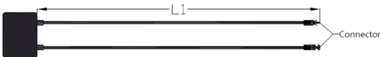
Fig. 7 (1) The full-cell module junction box
